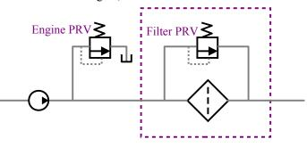
If you lose lubrication, you also lose bearings. The PRV in the filter is either a leaf spring or a coil spring that pushes a disk of paper or rubber against a hole.
