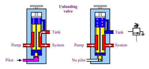
When the pilot pressure drops below a certain value, the spool is pushed down by the spring, and flow to the tank stops. All the flow goes to the system. The spool is hollow, so we can relieve the pressure above and below the spool as it moves up and down. The spring is adjustable, so we can set the required pilot pressure.
