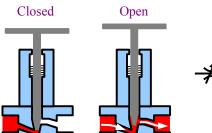
the throttle is  $p_1$ , shown in red. The pressure downstream is  $p_2$ , shown in blue. We want to maintain pressure  $p_2$ .
