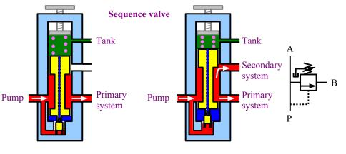
This symbol is a little different from the one in the book. The textbook symbol doesn't show both circuits, A and B. The increased pressure in the pilot line pushes the spool up, and opens flow to a secondary circuit, marked "B" on the hydraulic symbol. In the lab, circuit B is the second cylinder.
