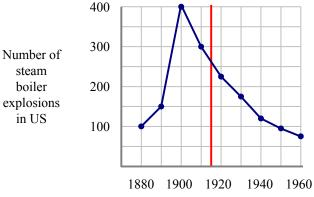
So what happened in 1915 that ensured a reduction in boiler explosions? The American Society of Mechanical Engineergs (ASME) published its famous *Boiler Code*, which establishes requirements for materials and dimensions of steam boilers. The *Boiler Code* is what put ASME on the map as a professional society.
