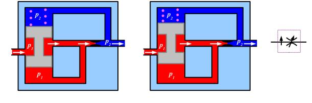
There are other types of valves that can compensate for pressure and temperature changes. This valve compensates for pressure. The fluid is flowing from left to right, past a spool, and through an adjustable throttle. The pressure upstream from
